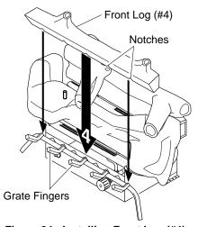
Figure 24 - Installing Front Log (#4)
